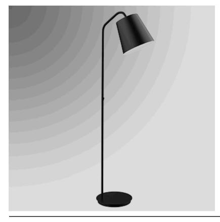
72" Matte Black Floor Lamp, medium base socket, on/off rocker switch on column at 40"AFF, 8' Black 45° cord, 8-3/8"x11-7/8"x11" Matte Black Metal Shade with Painted White Interior & Frosted White Acrylic Bottom Diffuser. Recommend 1100 lumen LED bulb.
